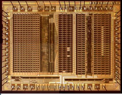
A built-in current monitor for  $I_{DDQ}$  testing is implemented in each block.
